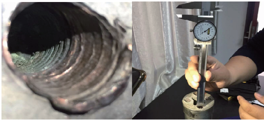
图 5 螺孔插入深度测量图 Fig. 5 Diagram of screw hole insertion depth measurement
