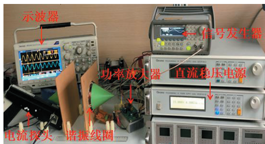
图 11 磁耦合谐振式无线电能传输实验平台 Fig. 11 Experimental platform for magnetically coupled resonant wireless power transfer
