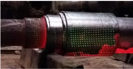
(c) 点阵结构光投射
