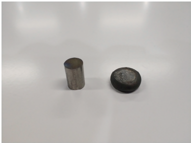
图 2 热压缩试样鼓度现象 Fig. 2 Bulge phenomenon of hot compression sample
